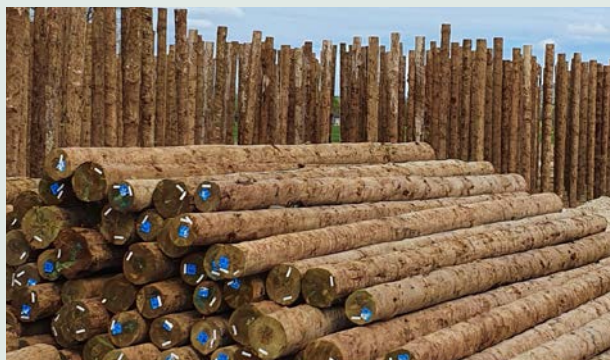
These TTT Uglies were joined during installation to reach a depth of 21.0m.
